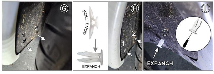
FIGURE J Logo-side of flap facing rear bumper, align to mounts 1 & 2. Loosely install SMWASH & 1SS#8 into mount 2.
