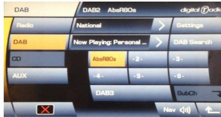
1) Press and hold the blank buttons “x-” on the DAB page for up to 2 seconds and this action will create a preset of that station to that number on the button.
