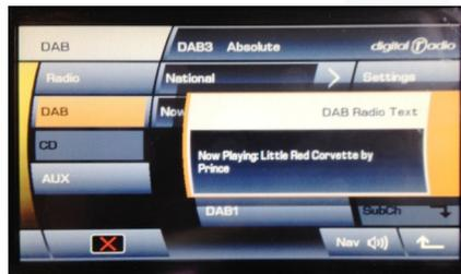
2) To display Dynamic Label Segment (DLS) being transmitted by the station. By pressing “>” on the display a pop up display will appear.
