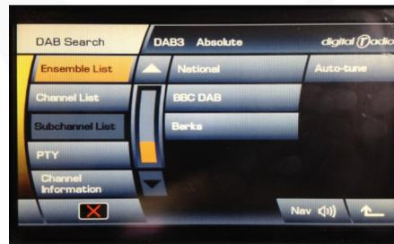
On first power up press **Auto-tune** button to scan for any digital radio stations that have been recognised by the digital receiver.
