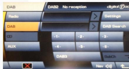
To select the preset station as part of the preset list. First skip through the stations using " " button on HU and once you find the station that you want to put in a pre-set list press and hold the blank buttons "x-" on the DAB page for up to 2 seconds and this action will create a pre-set of that station to that number on the button.
